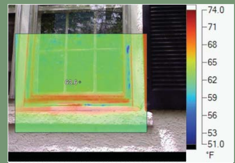
This infrared image taken on a cool day shows where heat (red) is escaping around a window that has poor air sealing.
