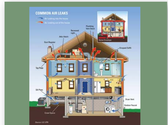
Air movement in your home: Hot air moves towards cold air. In the winter, warm interior air will be drawn towards colder areas and escape outside, drawing the cooler air inside.
